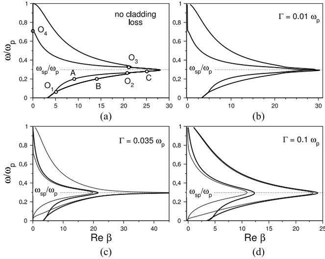
Fig. 3. Dispersion diagrams showing frequency versus the real part of the propagation constant for negligible cladding losses (a) and for three different cases of low, moderate and high loss (b)–(d). Labels A, B, C on subfigure (a) correspond to modes showed in Fig. 2.  $O_1$ – $O_4$  are exceptional points.
