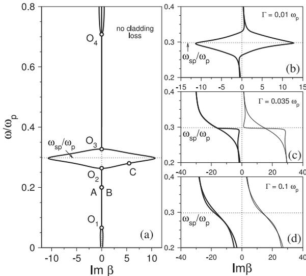
Fig. 4. Dispersion diagrams where frequency is plotted versus imaginary part of propagation constant for the non lossy case (a) and for the three different cases corresponding to low, moderate and large loss (b)–(d). Labels A, B, C on subfigure (a) correspond to modes showed in Fig. 2.  $O_1$ – $O_4$  are exceptional points.
