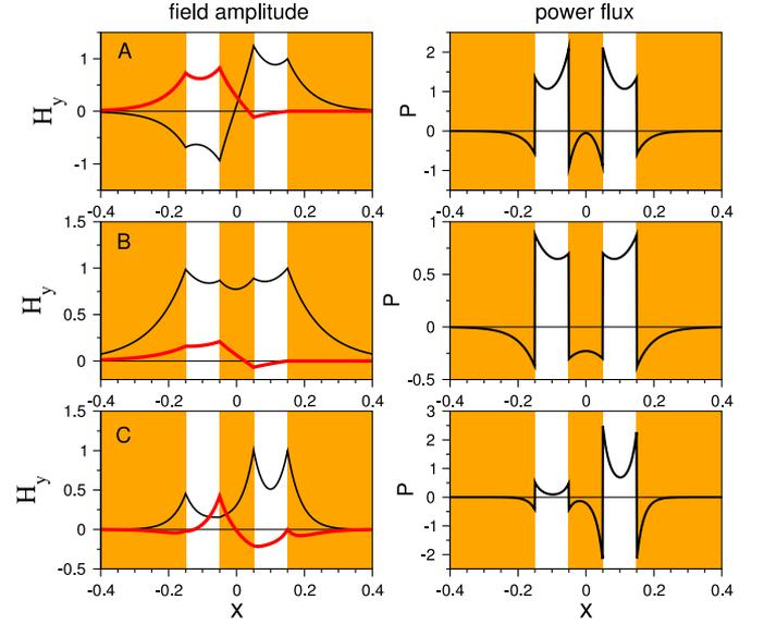
Fig. 2. Some examples of the complex modes. On the left column the real (thin black line) and imaginary (thick red line) parts of the magnetic component is plotted for three different modes. On the right column it is plotted the power flux for the same respective modes. Labeling letters correspond to the points in Figs. 3(a) and 4(a).
