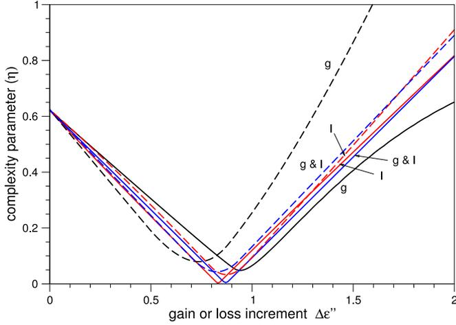
Fig. 5. Complexity parameter for different values of the gain/loss asymmetry. Line labels indicate the cases of increasing gain at the second core (label “g”, black line), decreasing loss at the first core (label “l”, red line) and the combination of both actions (label “g & l”, blue lines), but introducing half the effect at each of the cores. Continuous lines are for the symmetric mode and dashed lines for the antisymmetric mode.
