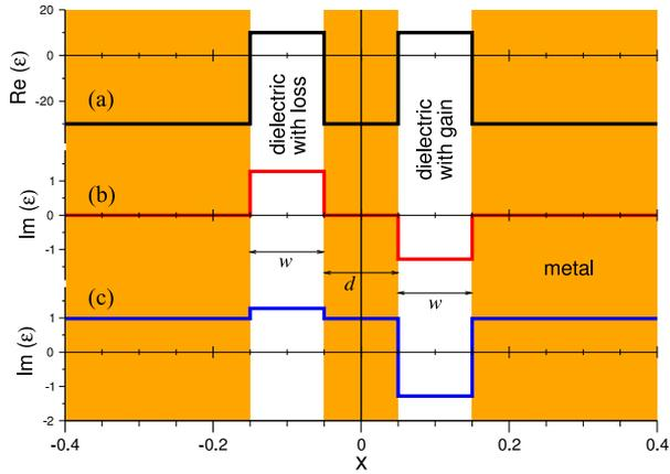
Fig. 1. A sketch of a directional coupler with metallic cladding (shaded) and dielectric cores. Overprinted are the dielectric functions: (a) real part, (b) imaginary part for vanishing cladding losses, and (c) imaginary part for realistic cladding losses.
