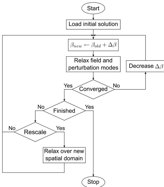
Fig. 2. Flowchart of the numerical adaptive procedure to track the perturbation eigenvalues in the linear stability analysis.
